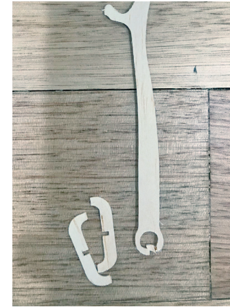
Figure 5.d: We found that Balsa wood can break easily, hence we discarded it.
