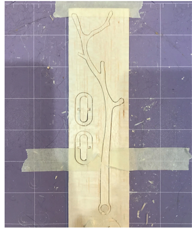
Figure 5.c: We used a Cricut machine to cut balsa wood in an organic twig shape.
