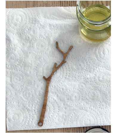
Figure 5.e: Finally we settled on the laser-cut bamboo twig as the stirrer and used tung-oil to waterproof it.
