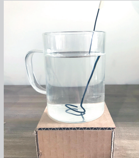
Figure 4.c: Addition of metal rod increased the sound volume but sound was not consistent.
