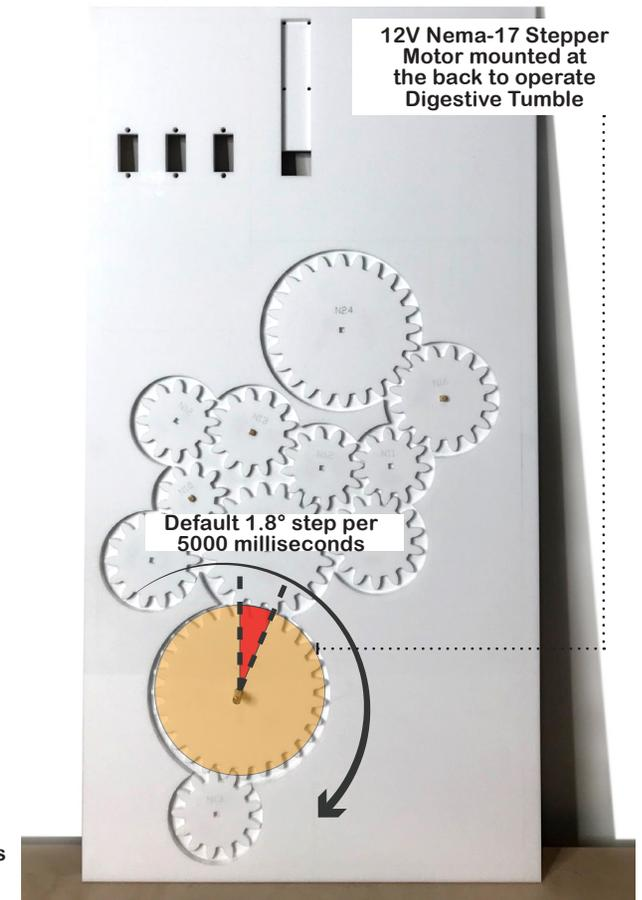
**Figure 8:** Digestive Tumble represents the digestion rate of different meals through a stepper motor.
