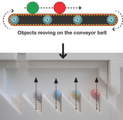
**Figure 11:** Fermentation module utilizes a zig-zag conveyor belt to move beads.
