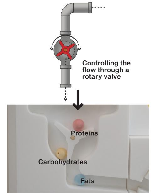
**Figure 17:** Swallowing module utilises a rotary mechanism to control the flow of beads.
