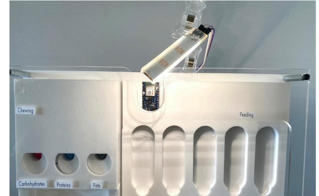
**Figure 20:** Digestive Tumble is attached with an LED light to provide consistent lighting to the BLE sensor.
