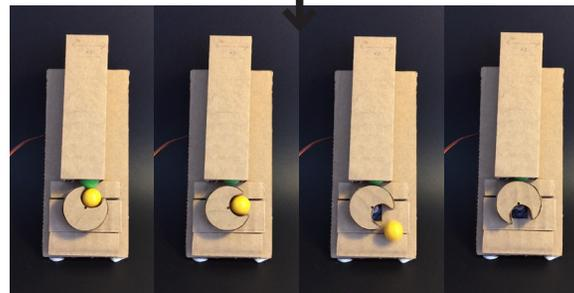
**Figure 12:** Chewing module uses the hold and release mechanism to release beads.
