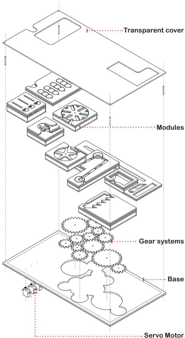
**Figure 19:** Digestive Tumble follows a minimalistic design, and utilises 12 various sized gears and 1 stepper motor to run all nine modules. The system is attached with a transparent cover to avoid spilling of beads and tokens and to keep all the modules intact.
