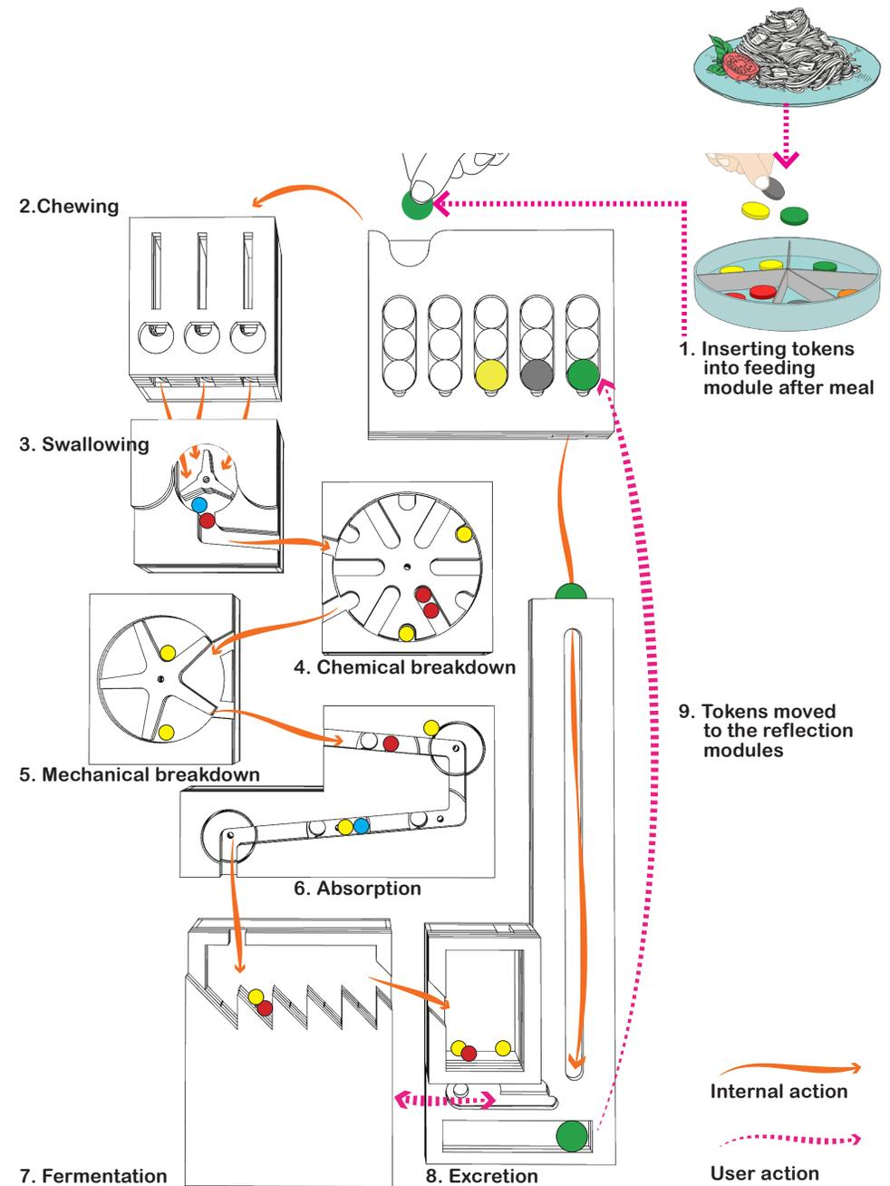
Figure 3: Diagram shows how the tokens and beads traverse through each module.
