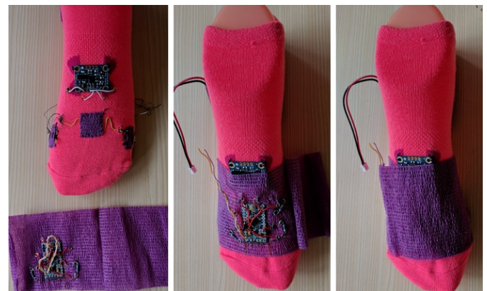
Figure 6: Most of the electronic components like Arduino board and resistors were placed on an external cloth. This arrangement helped in developing both comfortable and stretchable sock prototype.
